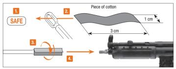
Prepare a thin rod with a length of approx. 30 cm. Attach a piece of cotton fabric to its end and clean the barrel with some silicone oil.
